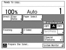
When toner runs out completely and prints can no longer be made, the message <Replace the toner.> appears on the touch panel display. Pressing [Recover Later] enables you to continue operations. However, you have to replace the toner cartridge to make further prints.
